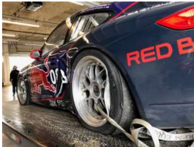
Picture of left side after being hit while racing at COTA. Note both rims flattened by impact falling back to track. Car felt like it was 30 deg off of horizontal before gravity took over.
