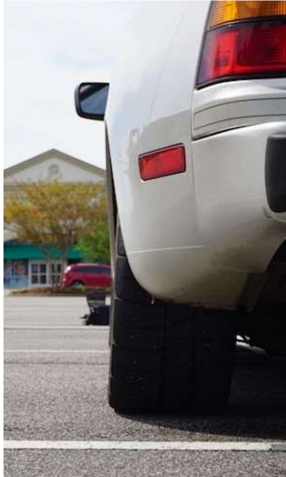
Rear tire slanting inward at top = negative camber.
